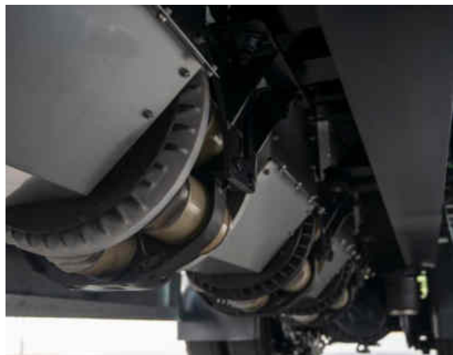
Eddy current brakes with air ducts
